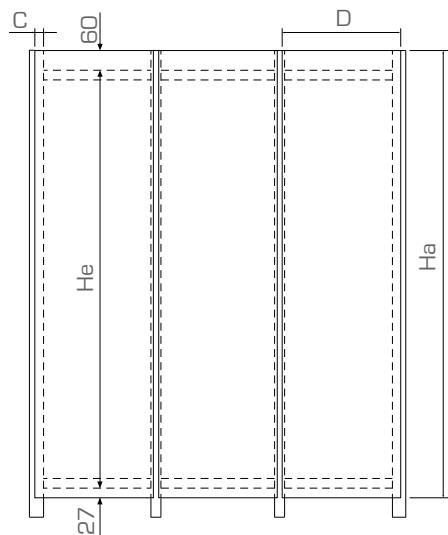
$$\begin{aligned} \textcircled{1} \quad \text{Ha} &= \text{He} + 60 + 27 \\ \textcircled{2} \quad \text{X} &= \text{C} + 74 \\ \textcircled{3} \quad \text{Y} &= \text{D} - (\text{Z} + \text{X}) \\ \textcircled{4} \quad \text{Z} &= \text{D}/2 + 210 \\ \textcircled{5} \quad \text{X}' &= (\text{D} - 140)/2 \end{aligned}$$
