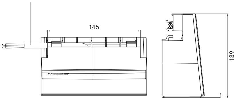
Fig.: Dimensioni in mm
