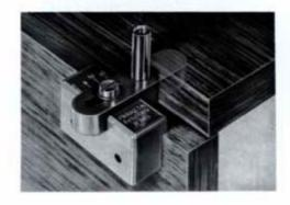
Example for template drill set B 580 for quick mounting cabinet hinge 580.
